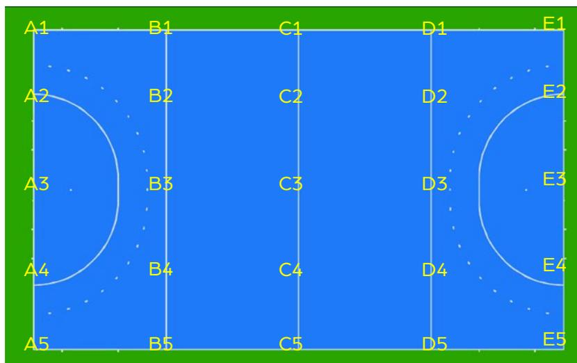
Figure 3 – grid positions for measuring field profile & gradients
