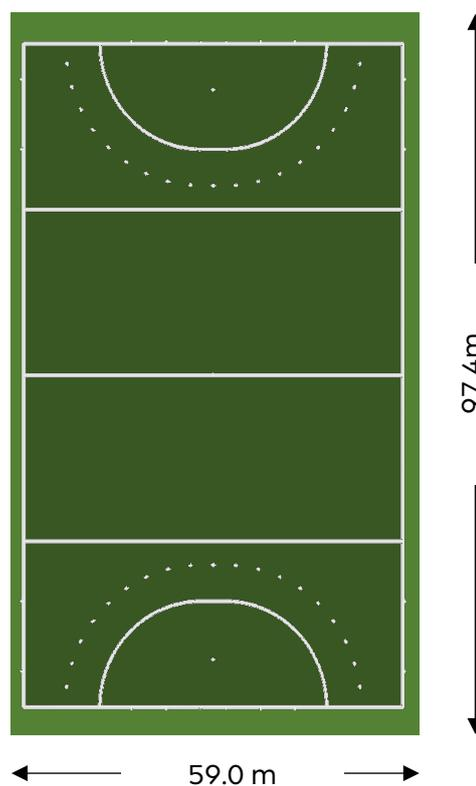
Field with Minimum Run-offs. Inner run-off in hockey turf, outer run-off hard paving
